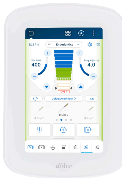
The integrated Midwest apex locator accurately identifies—and shows—the file position relative to the canal apex on the DS7 touchscreen as you work.
